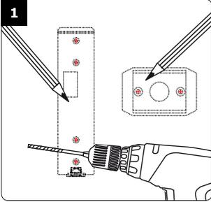
Verify the distance between the PROFIL100EC keypad and its remote electronic (refer to page 3, Notes and Recommendations). Place the back plate of the PROFIL100EC on the wall and the bracket of the remote electronic then mark with a pen the hole location then drill the 2 mounting holes (5mm drill bit  $\varnothing$  and 35mm hole depth) and the hole wiring access.
