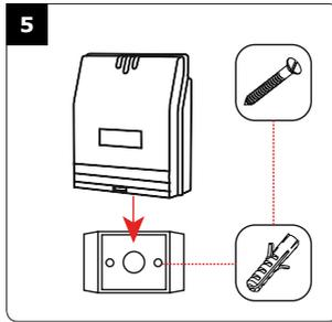
Insert the 2 plastic anchors in the holes. Place the bracket of the electronic and screw on the wall using the supplied M4x30 screws. Slide the box from up to down on the bracket.
