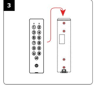
Insert the cable in the hole access area of the back plate. Then mount the keypad on the back plate, placing first the top in the hooks and then the bottom.
