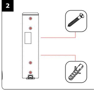
Insert the 2 plastic anchors in the holes. Mount the back plate of the PROFIL100EC with the (M4x30) mounting screws.
